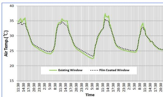
Fig. 8 Temperature in Insulation Box
